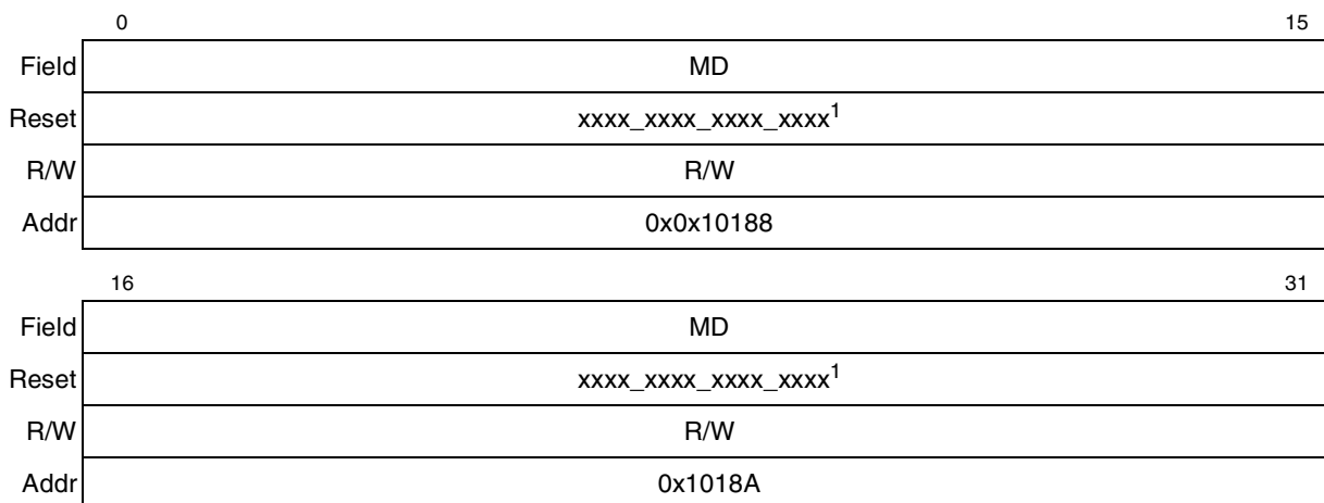
Figure 11-12. Memory Data Register (MDR)
